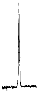
Fig. 9. Peak of 1 \mu l (0.73 mg) of n -decane obtained on the HPLC-IR detector system. For chromatographic conditions see Fig. 6. Detector conditions: wavelength, 3.46 \mu m; slit, no. 2; range, 1A; time constant, 4 sec.
